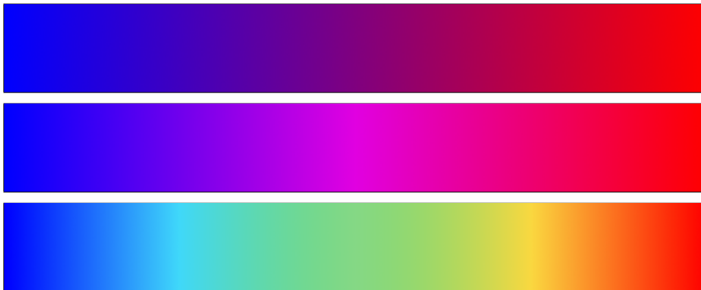
Figure 3: Examples of linear gradients. RGB space(top). HSL space: anti-clock-wise (middle) and clock-wise (bottom).
