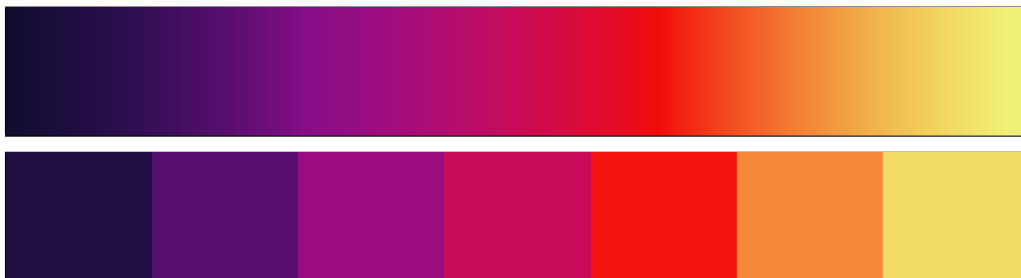
Figure 4: Example of a palette obtained from the discretization of a gradient in seven steps.
